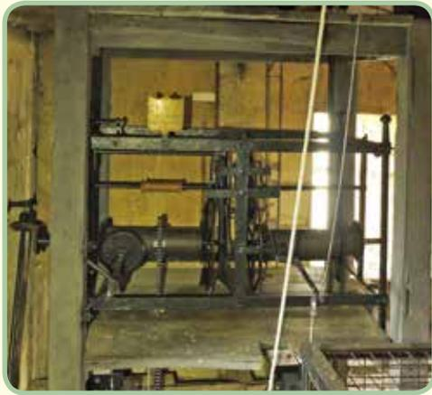
The 17th century clock in **St Peter's Church in Haresfield** has been repaired and given an electric winding mechanism, with help from GHCT. It had been silent for more than 30 years.
